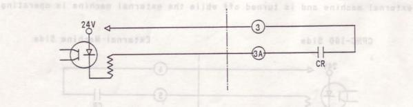
Switching between N.O (Normally Open) and N.C (Normally Closed) can be made by setting PA18. Turns at eldat and dolde to langis nolliang a emittunion hadk
