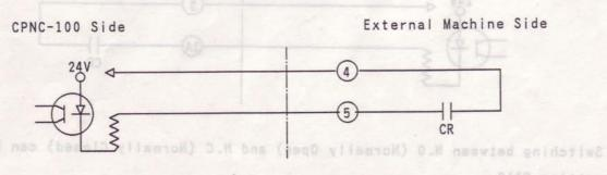
When outputting a position signal at which the table is returned after completion of automatic cycle of an external machine by a limit switch.
