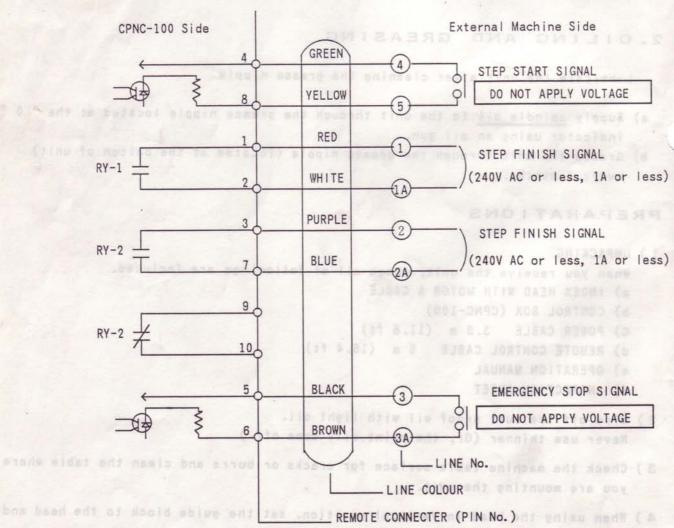
When line 4 and line 5 are on, the index head makes one step of indexing and will make the step finish relay (RY-1, RY-2) ON after finishing indexing, however,
