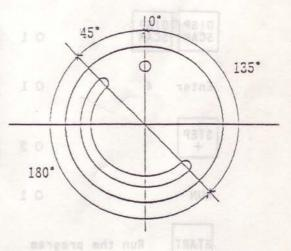
\*After moved to 45° making 180° cutting feed and then indexes 135°.
