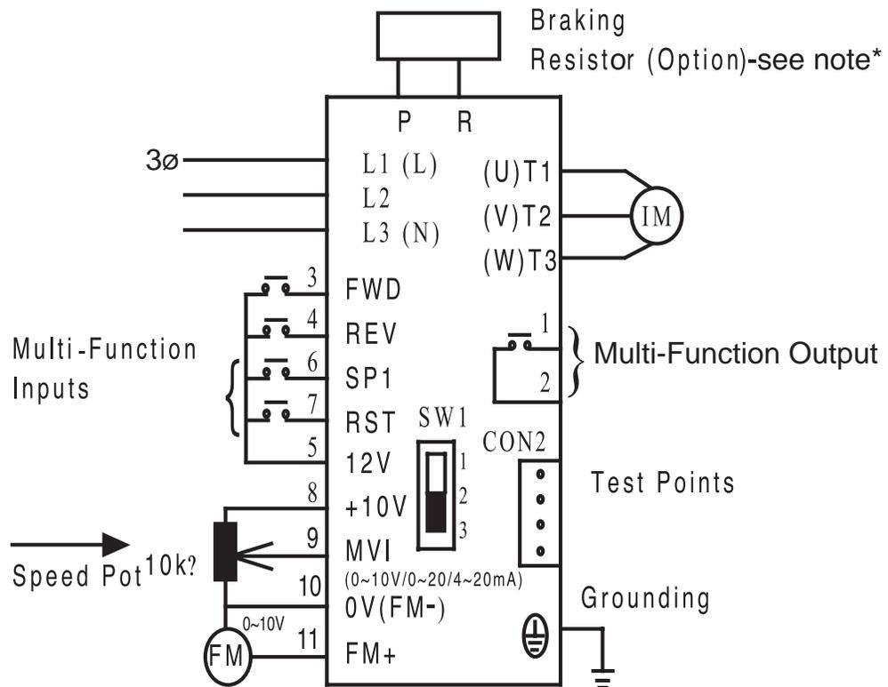
Wire Terminations to the AC drive must be made with either UL listed field wiring lugs or UL listed crimp type ring terminals.
