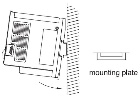
First place the groove on the back of module on the upper edge of din rail, then push the module down to lock-up position. Finally press the mounting plate upward into module.
