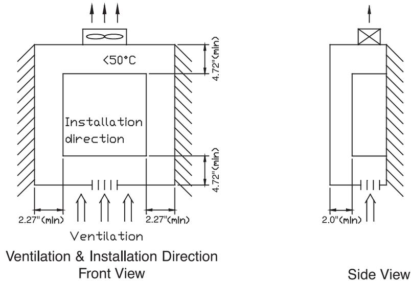
**Note:** Maximum temperature in the enclosure is 122°F (50°C) with Shield Sticker removed
