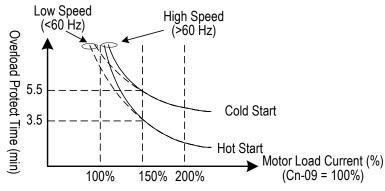
Fig. 36. Motor overload protection curve (Cn-09 setting = 100%)
