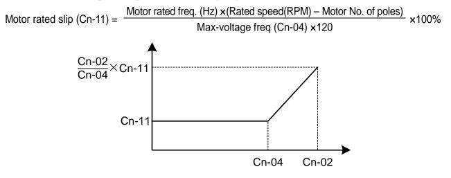
Fig. 19. Slip compensation limit
