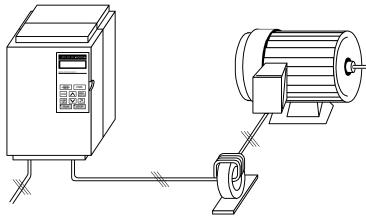
Note: All the line wire of U/T1, V/T2, W/T3 phase must pass through the same zerophase core in the same winding sense.
