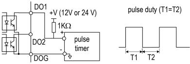
Fig. 45. Pulse signal output
