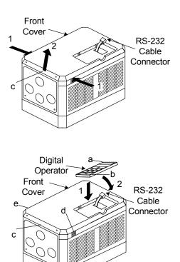
Mounting the front cover and digital operator
