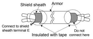
Fig. 3. Processing the ends of twisted-pair cables
