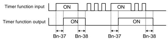
Fig. 15. An operation example of timer function
