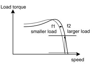
Fig. 18. Output frequency with slip compensation.
