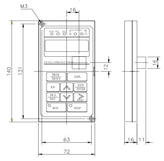
Fig. 6. LCD Digital Operator Dimension
