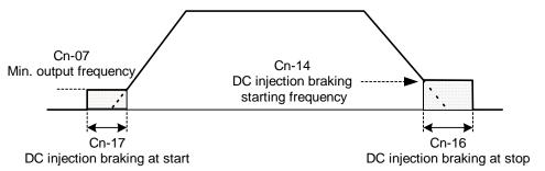
Fig. 20. DC injection braking time chart
