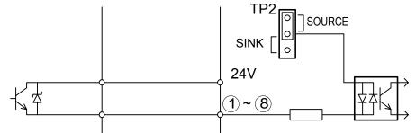
• PNP Sensor (Source) used for operation signal.
