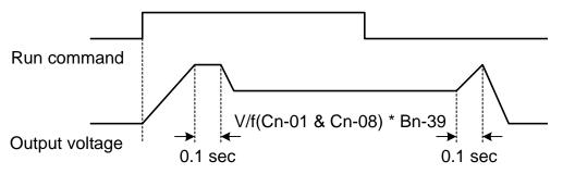
Fig. 16. Time chart for energy-saving operation
