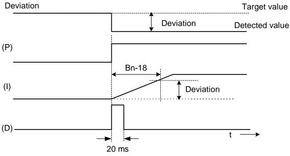
Fig. 13. Response of PID control for step-shape (deviation) input
