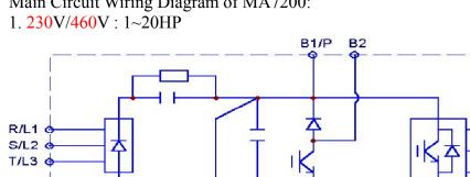
Main Circuit Wiring Diagram of MA7200:
