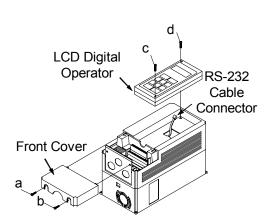
Attach the digital operator and tighten the screws in the place c and d. Insert the tabs of the upper part of front cover into the groove of the inverter and tighten the screws in the place a and b.
