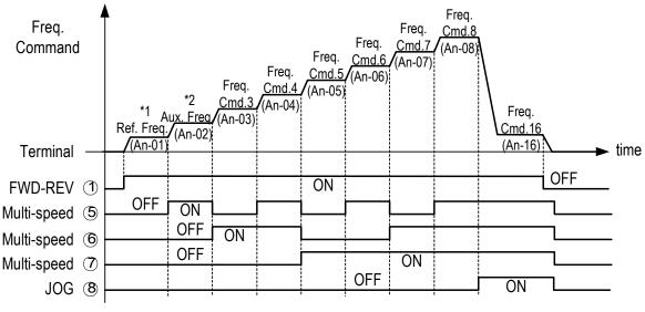
Fig. 40. Time chart for multi-step speed and jog command
