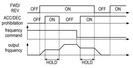
Fig. 41. Acceleration and deceleration ramp hold
