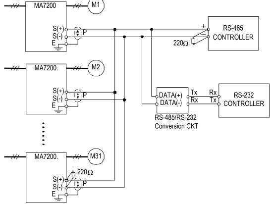
Fig. 50. Wiring for MODBUS Protocol Communication
