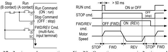
Fig. 37. 3-wire mode connection Fig. 38. Operation sequence in 3-wire mode diagram
