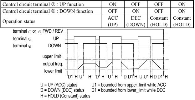
Fig. 44. Time chart of output frequency with the UP/DOWN function
