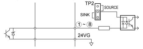
• NPN Sensor (Sink) used for operation signal.
