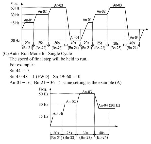
•  $Sn-44 = 1 \sim 3$ : If the inverter stops and re-starts again, it will continue running from the unfinished step, according to the setting of Sn-44.
