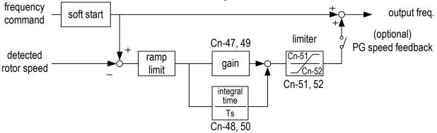
Fig. 43. PG speed control block diagram
