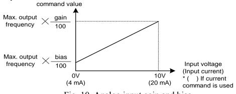
Fig. 10. Analog input gain and bias
