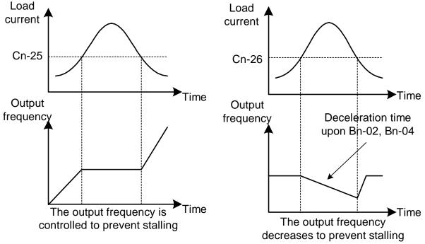
Fig. 23 Acceleration stall prevention function
