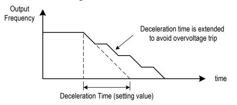
Fig. 34. Stall prevention function during deceleration (Sn-15= 1)
