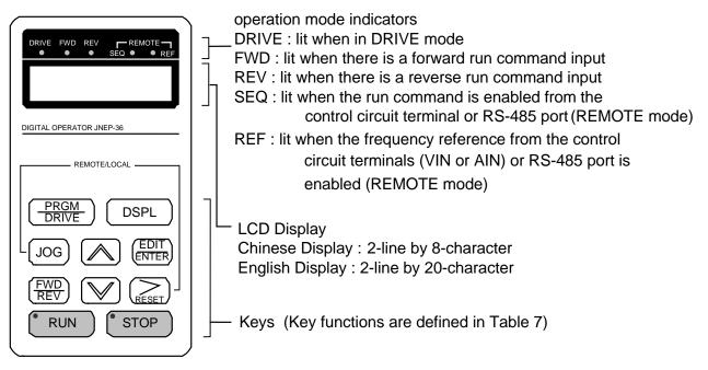
Fig. 8. LCD Digital operator
