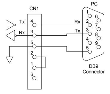
Fig. 52. RS232-C Typical Connection Diagram
