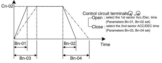
Fig. 9. Acceleration and Deceleration time
