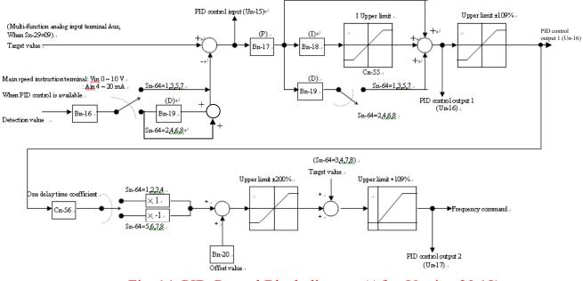
Fig. 14. PID Control Block diagram (After Version 30.18)
