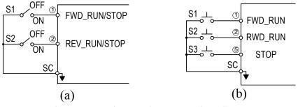
Fig. 39. 2-wire mode connection diagram
