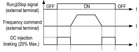
Fig. 35. Zero speed braking operation selection
