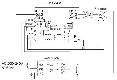
Fig. 49. Wiring of PG feedback
