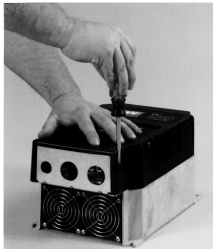
Figure 8: Removing Cover From 7.5 to 20 HP Inverters
