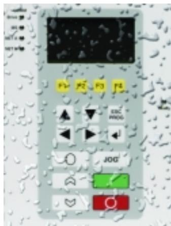
*The LCD display on the NEMA 4X SP600 is protected from the environment by the front cover overlay. The light emitting diodes LED modules on the new SP600 drive cover provides a visual indication of network operations, without having to open the cover.*
