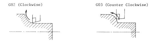
The position of the arc center is specified by using the address I in the X-axis (with radius value) and the address K in the X-axis.
