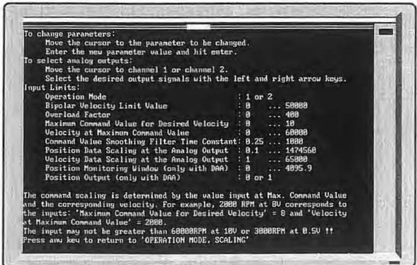
Fig. 43: "OPERATING MODES, SCALING"; help text for feedback versions with absolute encoder options
