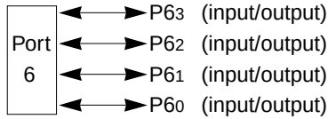
Figure 9-18 Port 6 Pin Functions in Modes 7, 2, and 1
