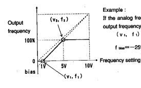
Example: If the analog frequency setting voltage is 1 to DC 5V and the output frequency is weighted to 0 to 100%, then:
