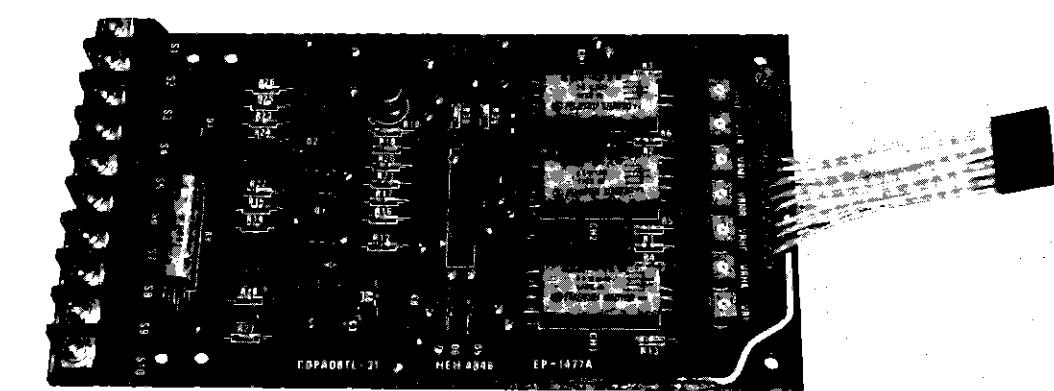
Torque limiter • Current limit pattern generate P.C.B.
