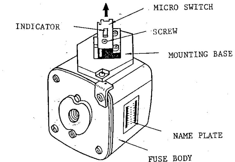
The fuse is connected between S.C. power source, U, V, and W phase, and thyristor in series to protect the thyristor from heavy current. If the fuse is blown out, indicator of micro switch installed at the top of the fuse body shows trouble. In above case, you have to change the fuse. Though the fuse is pushed on the mark, it is of no use against blowing off. (When changing fuse, please make sure current and type of fuse appeared on label covered fuse body).
