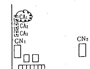
Make short circuit the pins CA<sub>1</sub> with a jumping wire as illustrated on the left.
