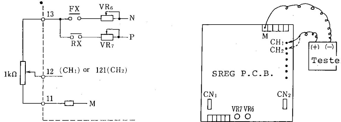
When the power supply for speed setting is illustrated above, the fine adjustments of max. speeds are regulated with VR<sub>6</sub> for forward and VR<sub>7</sub> for reverse.
