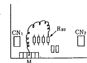
Make short circuit with the jumping wire between the end of R80 and the M terminal as illustrated on the left.
