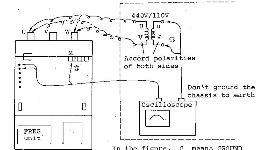
Example. The connection shows confirmation of a V phase pulse with real lines (With dotted lines shows a X phase pulse.)
