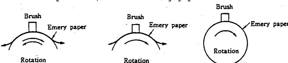
(A) Both direction (B) Single direction (C) Small D.C. motor
