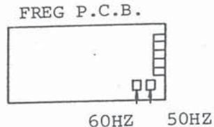
To change over the switch for 50 or 60 Hz frequency using, replace the mini jump socket from one side to another (The mini jump socket, what is called a switch, is used for frequency changing).
