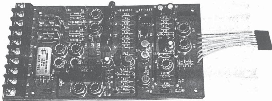
Torque limiter • Load meter P.C.B.
