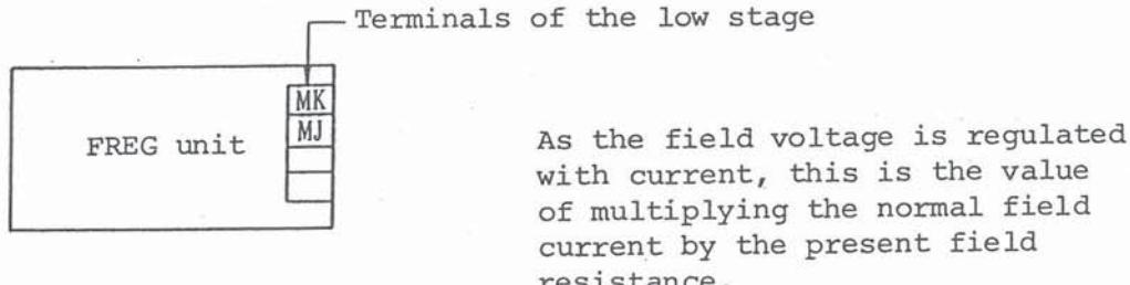
Don't touch the regulating volume resistance  $VR_4$  on the FREG P.C.B. despite the difference, 10 to 30% of the voltage between hot and cold conditions.
