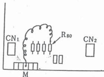
Make short circuit with the jumping wire between the end of R80 and the M terminal as illustrated on the left.
