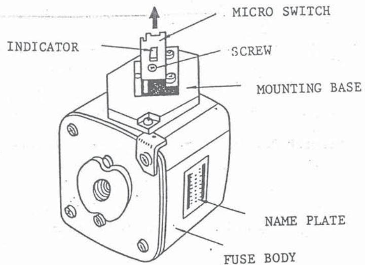
The fuse is connected between S.C. power source, U, V, and W phase, and thyristor in series to protect the thyristor from heavy current. If the fuse is blown out, indicator of micro switch installed at the top of the fuse body shows trouble. In above case, you have to change the fuse. Though the fuse is pushed on the mark, it is of no use against blowing off. (When changing fuse, please make sure current and type of fuse appeared on label covered fuse body.
