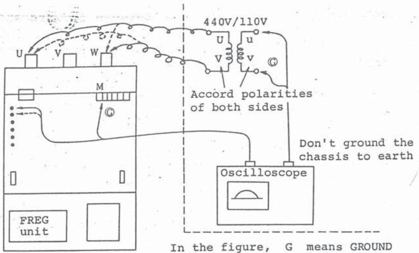
Example. The connection shows confirmation of a V phase pulse with real lines (With dotted lines shows a X phase pulse.)
