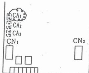
Make short circuit the pins  $CA_1$  with a jumping wire as illustrated on the left.
