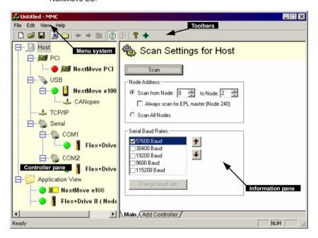
Figure 45 - The Mint Machine Center software
