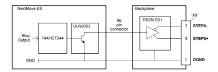
Figure 40 - Stepper output - STEP0 output shown
