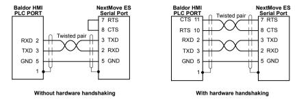
Figure 17 - RS232 cable wiring
