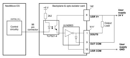
Figure 38 - Digital output circuit (DOUT0-7) with 'NPN' current sinking module - DOUT0 shown
