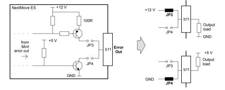
Figure 12 - Error Out level configuration
