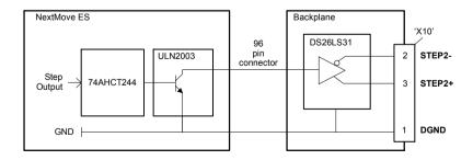
Figure 24 - Stepper output - STEP2 output shown
