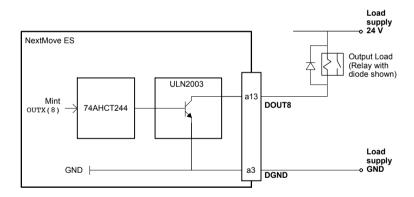
Figure 11 - Digital outputs (DOUT8-11) - DOUT8 shown
