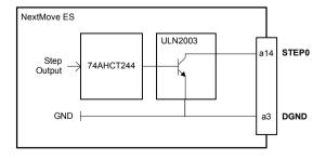
Figure 13 - Stepper output - STEP0 output shown
