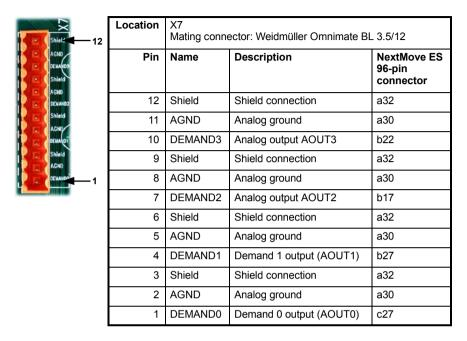
The outputs on the backplane are connected directly to the NextMove ES and do not pass through any circuitry on the opto-isolator card. See section 4.3.2 for electrical specifications and how to connect an output to a typical drive amplifier.
