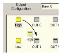
If you are going to use the error output, drag the Relay0 icon to the grey Drive Enable OP icon on the right of the screen.
