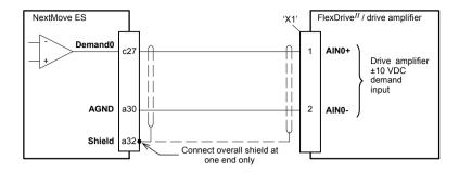
Figure 6 - Analog output - typical connection to a Baldor  $\mathsf{FlexDrive}^{II}$ ,  $\mathsf{Flex+Drive}^{II}$  or  $\mathsf{MintDrive}^{II}$
