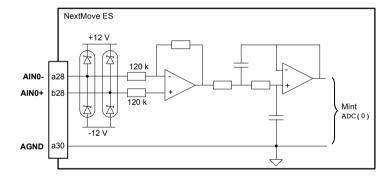
Figure 1 - Analog input, AIN0 shown
