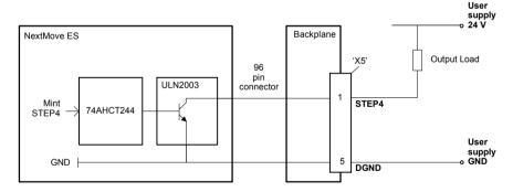
Figure 44 - Stepper output - STEP4 shown
