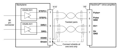
Figure 26 - Stepper output STEP2 - typical connection to a Baldor FlexDrive  $^{II}$ , Flex+Drive  $^{II}$  or MintDrive  $^{II}$
