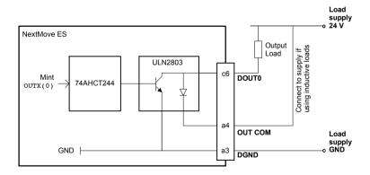
Figure 10 - Digital outputs (DOUT0-7) - DOUT0 shown
