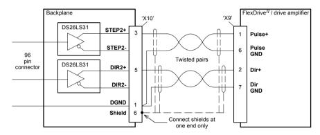
Figure 43 - Stepper output STEP2 - typical connection to a Baldor FlexDrive  $^{II}$ , Flex+Drive  $^{II}$  or MintDrive  $^{II}$
