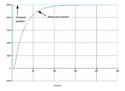
Figure 50 - Overdamped response
