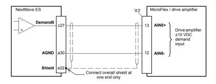
Figure 5 - Analog output - typical connection to a Baldor MicroFlex
