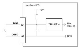
Figure 7 - General purpose digital input - DIN0 shown
