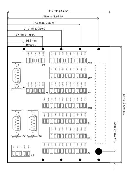
Figure 22 - Backplane BPL010-501 connector layout and dimensions
