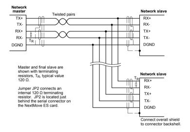
Figure 16 - 4-wire RS422 multi-drop connections
