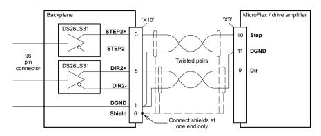
Figure 25 - Stepper output STEP2 - typical connection to a Baldor MicroFlex
