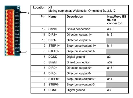
Stepper axes outputs 0-1 on the backplane are driven by DS26LS31 line drivers, providing RS422 differential outputs. See also Figures 42 and 43.
