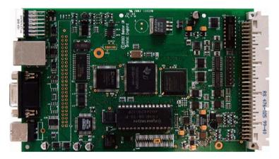
NextMove ES features the Mint motion control language. Mint is a structured form of Basic, custom designed for servo or stepper motion control applications. It allows you to get started very quickly with simple motion control programs. In addition, Mint includes a wide range of powerful commands for complex applications.
