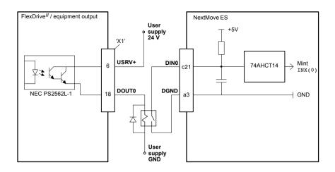
Figure 9 - Digital input - typical connections from a Baldor FlexDrive  $^{II}$ , Flex+Drive  $^{II}$  or MintDrive  $^{II}$
