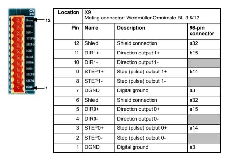
Stepper axes outputs 0-1 on the backplane are driven by DS26LS31 line drivers, providing RS422 differential outputs. See also Figures 25 and 26.
