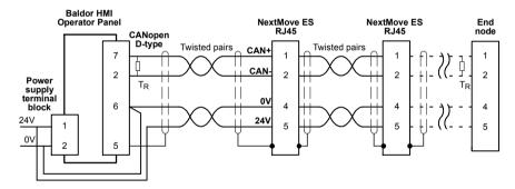
Figure 19 - Typical CANopen network connections
