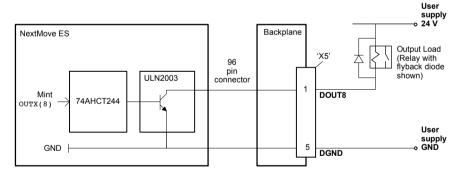
Figure 39 - Digital output circuit (DOUT8-11) - DOUT8 shown
