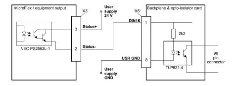
Figure 32 - Digital input - typical connections from a Baldor MicroFlex
