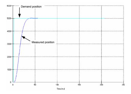
Figure 51 - Critically damped (ideal) response
