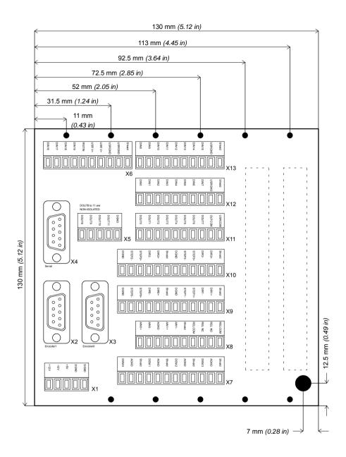
Figure 27 - Backplane BPL010-502/503 connector layout and dimensions
