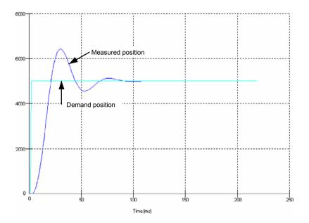
Figure 49 - Underdamped response
