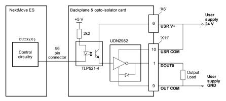
Figure 37 - Digital output circuit (DOUT0-7) with 'PNP' current sourcing module - DOUT0 shown
