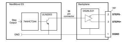
Figure 23 - Stepper output - STEP0 output shown
