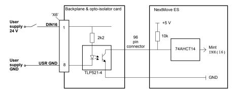
Figure 31 - Digital input circuit (DIN16) with 'active high' inputs
