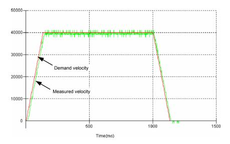
Figure 52 - Correct value of KVELFF
