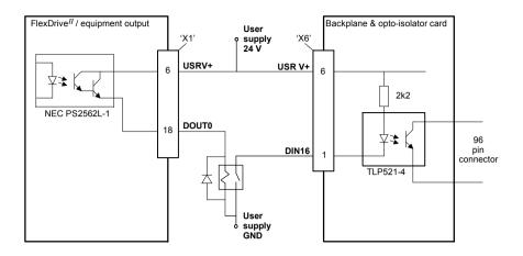
Figure 36 - Digital input - typical connections from a Baldor FlexDrive  $^{II}$ , Flex+Drive  $^{II}$  or MintDrive  $^{II}$
