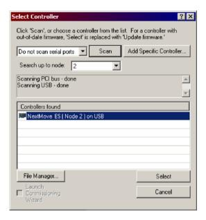
Note: If the NextMove ES is not listed, check the USB or serial cable between the NextMove ES and the PC. Check that the NextMove ES is powered correctly, and has completed its startup sequence (indicated by the node number being displayed by the Status display). Click **Scan** to re-scan the ports.
