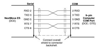
Figure 15 - RS232 serial port connections
