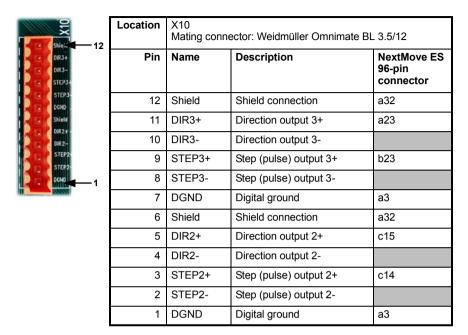
Stepper axes outputs 2-3 on the backplane are driven by DS26LS31 line drivers, providing RS422 differential outputs.
