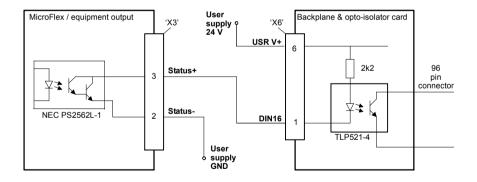
Figure 35 - Digital input - typical connections from a Baldor MicroFlex
