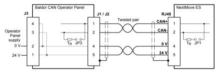
Figure 20 - Baldor CAN operator panel connections
