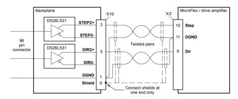
Figure 42 - Stepper output STEP2 - typical connection to a Baldor MicroFlex
