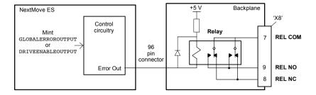
Figure 29 - Relay connections
