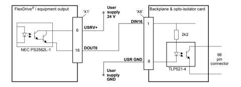
Figure 33 - Digital input - typical connections from a Baldor FlexDrive  $^{II}$ , Flex+Drive  $^{II}$  or MintDrive  $^{II}$
