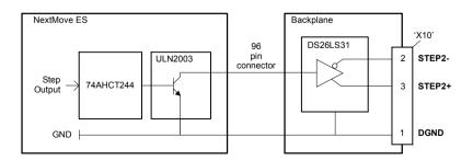
Figure 41 - Stepper output - STEP2 output shown
