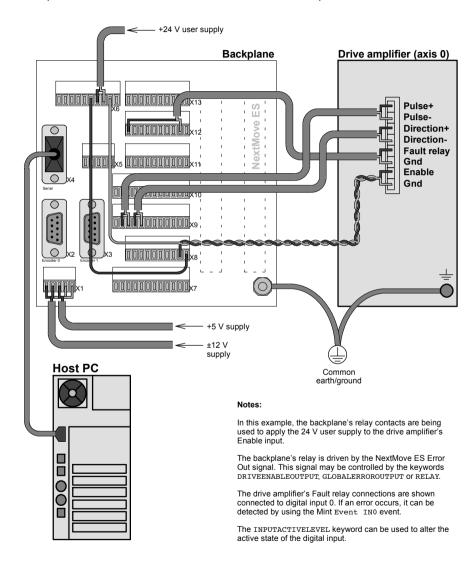
Figure 21 - Example minimum system wiring
