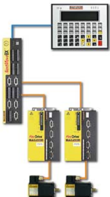
◀ A range of Human Machine Interface (HMI) panels are available from Baldor which can be interfaced via the CANopen port. With Mint's ability to perform motion and I/O tasks simultaneously, NextMove BX II is ideally suited as a complete machine controller.
