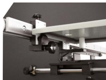
Alternating quick-clamping system for chamfers double ball optionally at the top or bottom.
