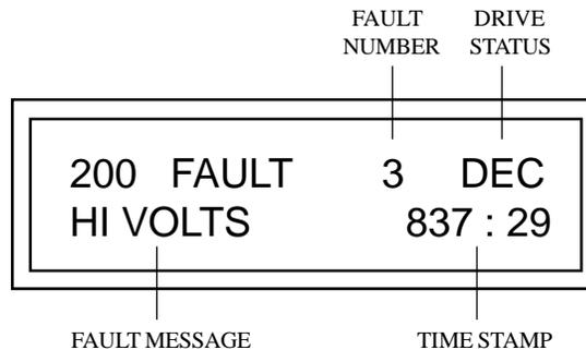
The above display indicates that the third fault was a HI VOLTS (abbreviation for HIGH DC BUS VOLTAGE) fault that occurred at 837:29 on the run time meter. The DRIVE STATUS portion of the display indicates that the drive was decelerating (DEC) when the fault occurred. Refer to Section 20.0 - TROUBLESHOOTING for a list of the possible fault messages that can appear on the display.
