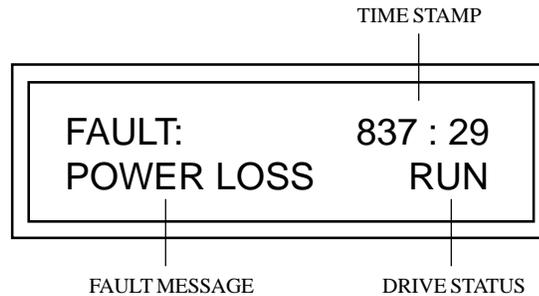
The fault display above indicates that the drive tripped on a POWER LOSS fault that occurred at 837:29 on the run time meter, and the drive was in a RUN state when it faulted. Refer to Section 20.0 - TROUBLESHOOTING for a list of the possible fault messages that can appear on the display.
