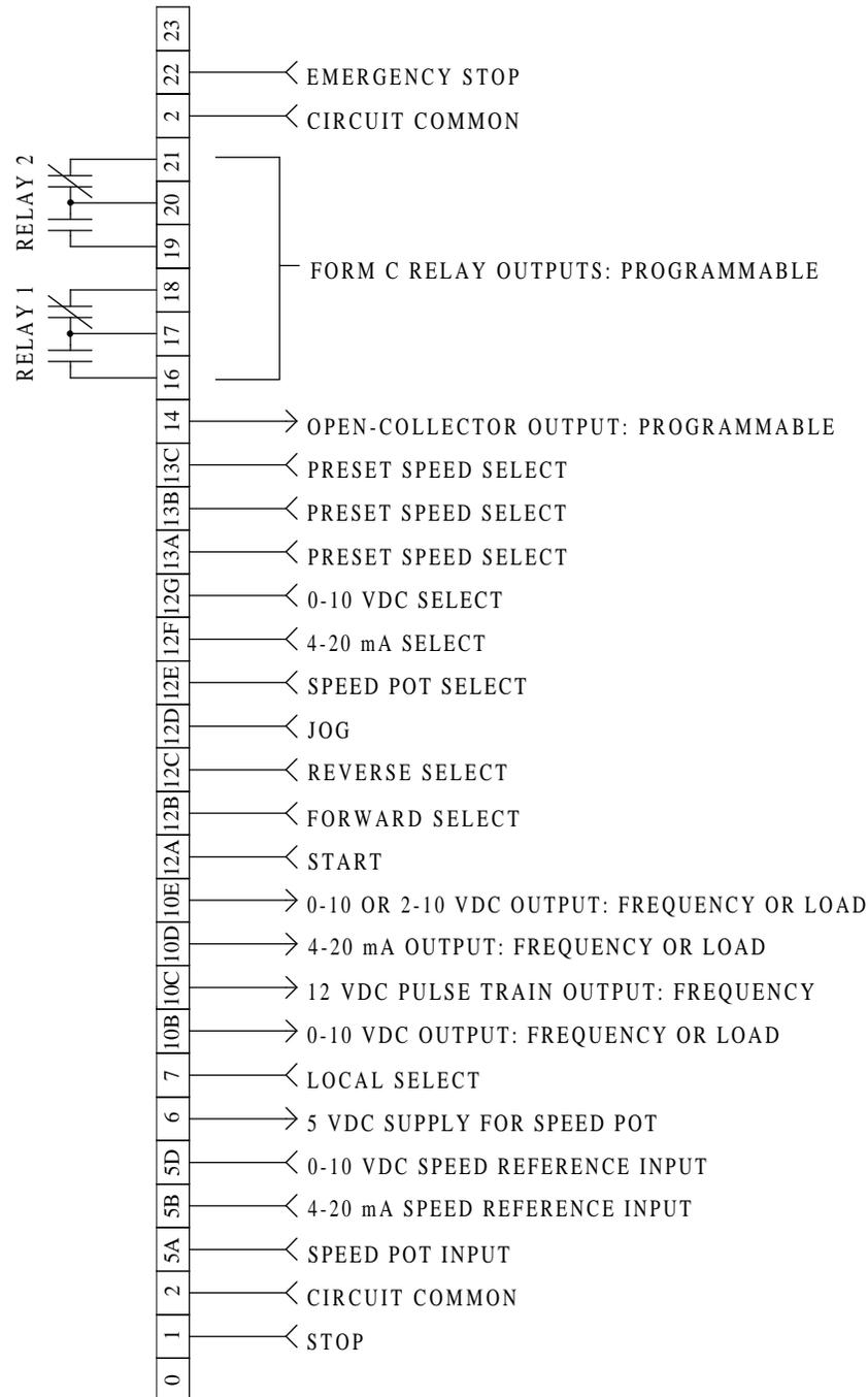
A complete description of operating the drive in the REMOTE mode can be found in Section 14.2. The following diagrams provide a quick reference for wiring the drive for the most common configurations.
