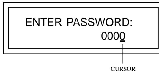
To enter the password, use the numeric keys to type in the password value and then press the ENTER key. If the ENTER key is pressed while the PASSWORD prompt reads 0000, the FAULT HISTORY (Parameter 200) display will be accessed, allowing an operator to view the FAULT HISTORY without knowing the password.
