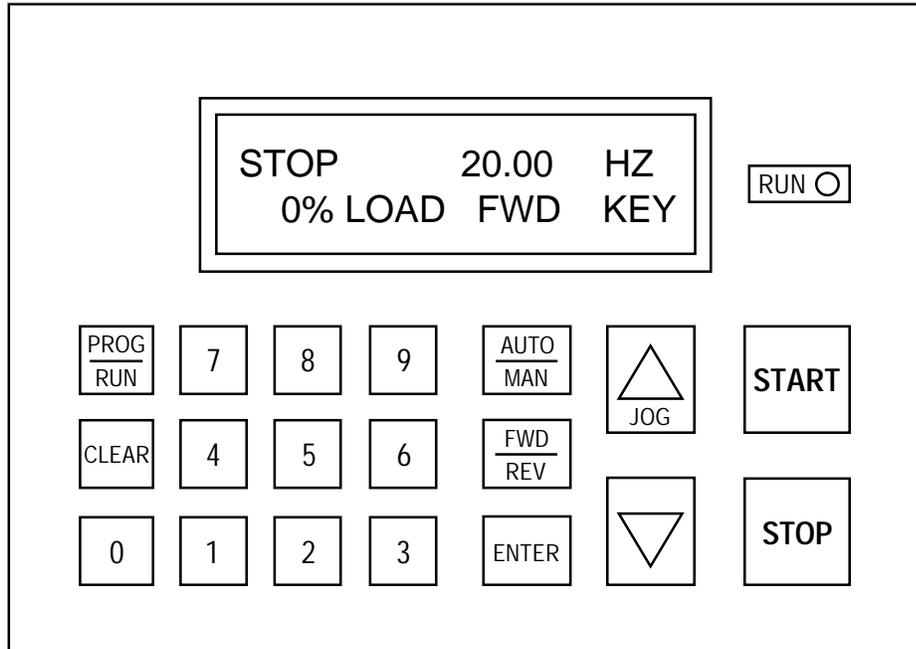
To program the drive, the PROGRAM mode must be entered by pressing the PROG/RUN button on the keypad. If the password protection is disabled, pressing the PROG/RUN key will result in direct entry into the PROGRAM mode. If the password protection is enabled, the PASSWORD prompt will appear when an attempt is made to enter the PROGRAM mode. The PASSWORD display appears as follows:
