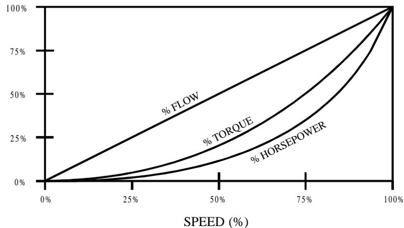
Variable torque refers to the fact that the torque required varies with the square of the speed. Also, the horsepower required varies with the cube of the speed, resulting in a large reduction in horsepower for even a small reduction in speed. It is easily seen that substantial energy savings can be achieved by reducing the speed of a fan or pump. For example, reducing the speed to 50% results in a 50 HP motor having to produce only 12.5% of rated horsepower, or 6.25 HP.
