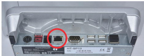
ECHO STATION ETHERNET PORT
