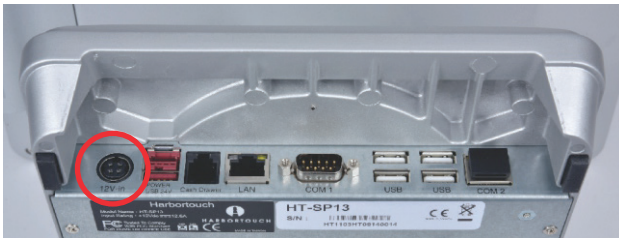
POWER CABLE PORT ON BACK OF ECHO STATION
