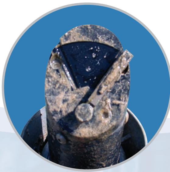
Despite significant bio-fouling after a 12 month deployment, the optical face of the DTS-12 is clean and perfectly operational.
