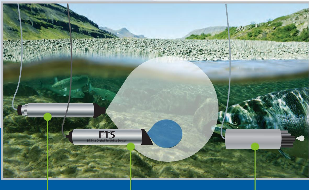
Typical single-parameter sensor has a large viewing volume that often intersects the surface and riverbed, generating false turbidities.
