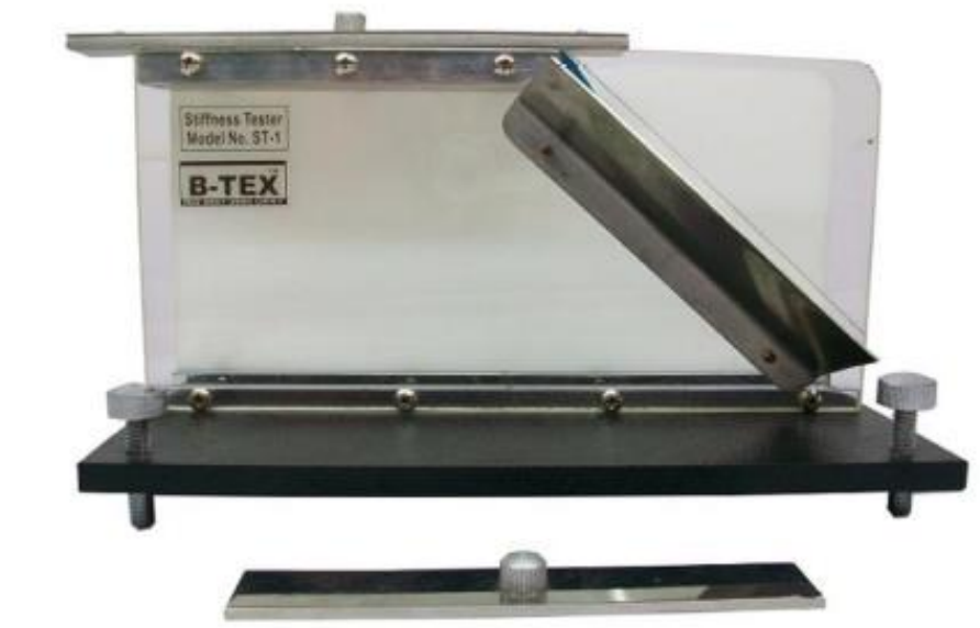
Figure 3: Shirley Stiffness Test Equipment
