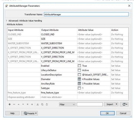
This image shows the Control Valve CAD feature, having its attributes mapped to the correct output field and domain definition.
