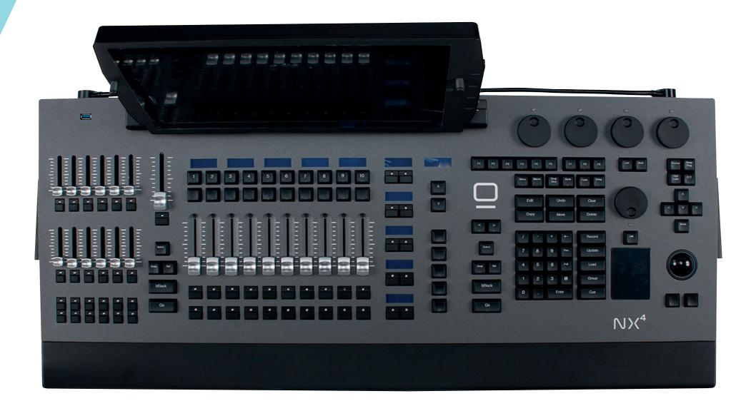
Two independent playback sections offer instant access. The main playback with 10 motorized faders plus 10 play-pairs allows for quick page changes while the sub playback with 12 faders and 12 button playbacks allows important cues to always be at the user's fingertips.
