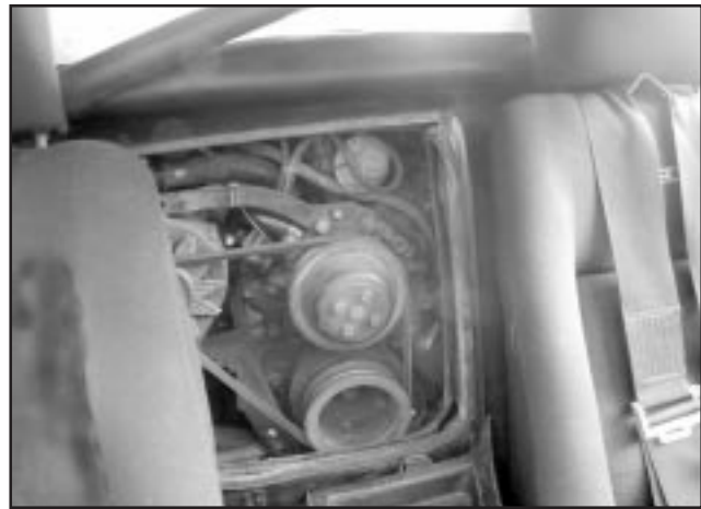
The removable fiberglass center section hangs on a sheetmetal lip and is held in place by rubber fasteners (both broken, unfortunately.) Apparently there was a removable sheetmetal firewall underneath, but this has gone missing, so the cabin gets hot and loud in a hurry!
