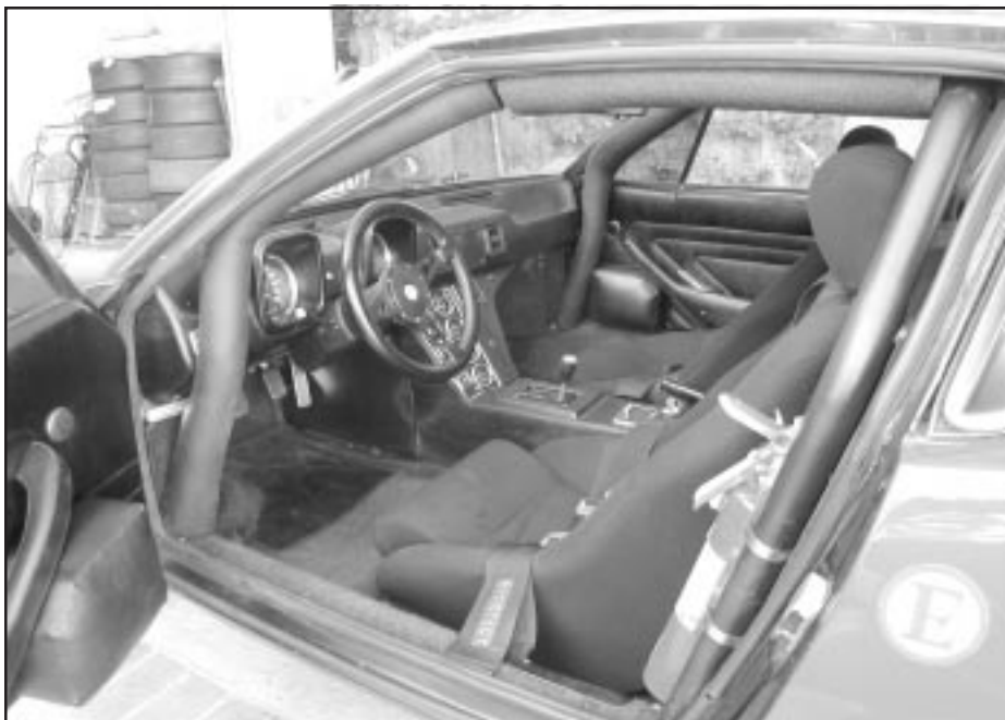
The interior is original except for the LeCarra steering wheel and Sparco racing seats. Note the padded knee bolsters on each door. The roll cage padding completely blocks access to the windshield wiper switches!
