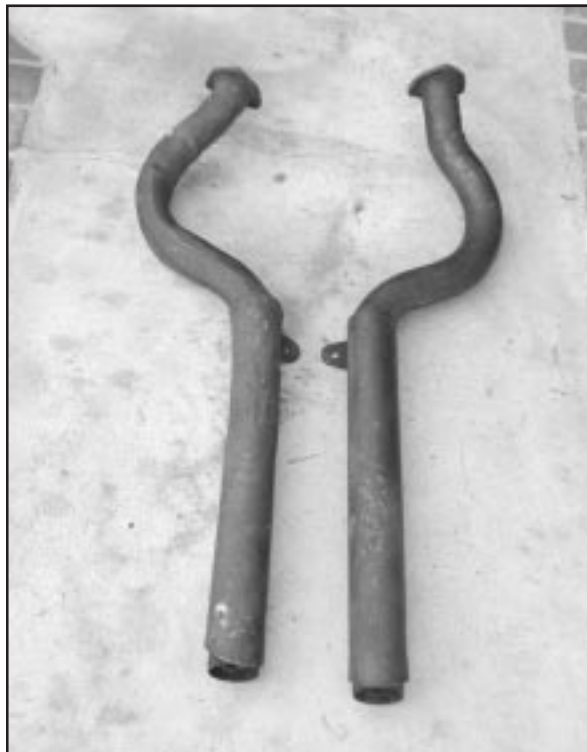
The original straight exhaust pipes had crude home-made silencers added
