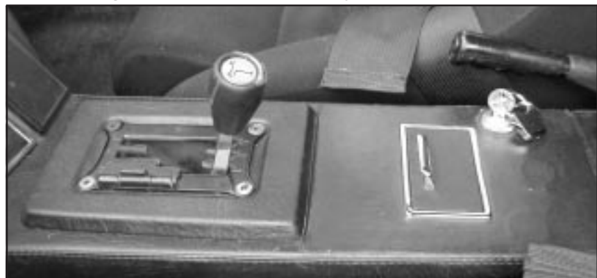
The shift gate has a hinged reverse lockout. The chrome shift lever has been shortened. The ignition switch was positioned in the cigarette lighter hole originally, and was apparently moved closer to the driver before finally being moved to its current location
