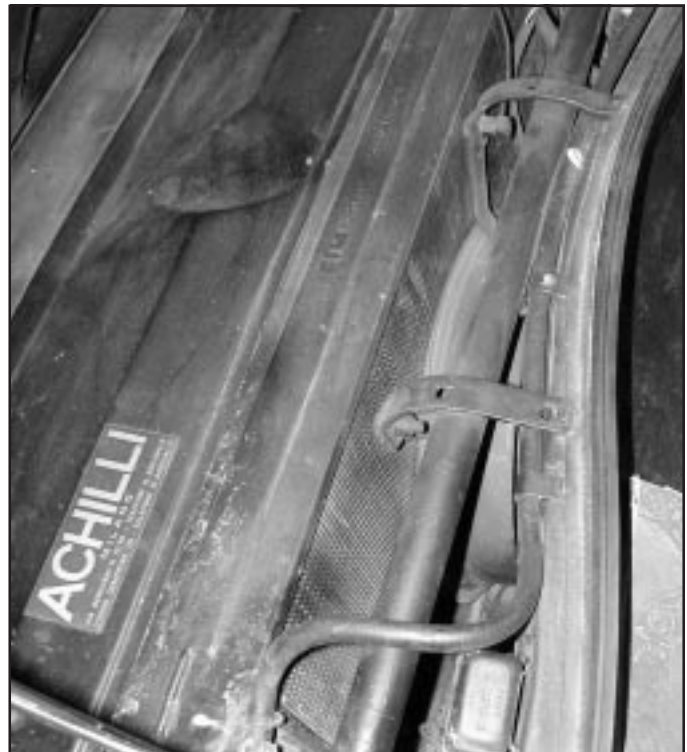
A third radiator fan was added, switched by a stock relay. The radiator is a standard, original unit
