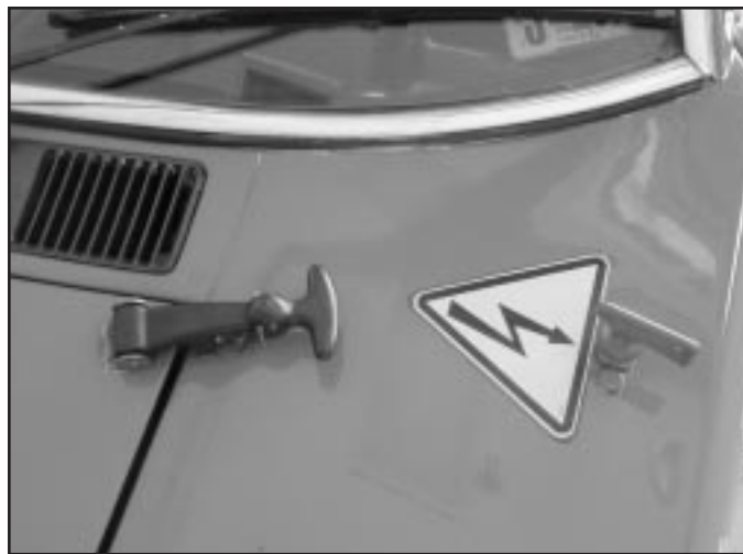
Rubber hold-downs supplant the stock hood and decklid latches. The original right-side battery shut-off switch is missing, and a replacement has been crudely bolted to the underside of the left fender
