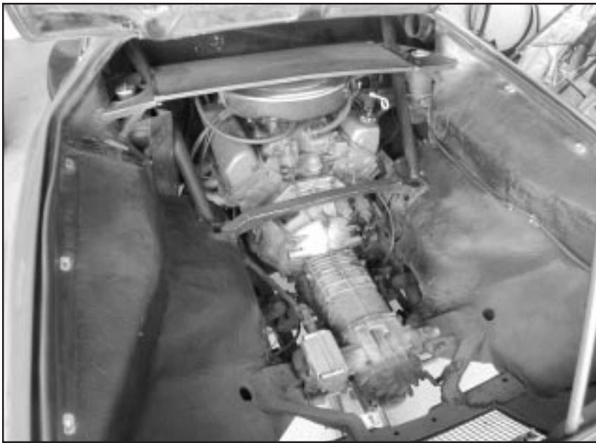
The engine is virtually stock except for the aluminum intake manifold and Holley carburetor. The roll cage requires the water bottles to be relocated, as it fights past the engine screen to bolt to the inner wheelhouses. The air conditioning system is missing
