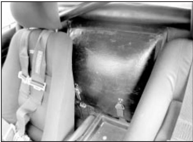
The removable fiberglass center section hangs on a sheetmetal lip and is held in place by rubber fasteners (both broken, unfortunately.) Apparently there was a removable sheetmetal firewall underneath, but this has gone missing, so the cabin gets hot and loud in a hurry!
