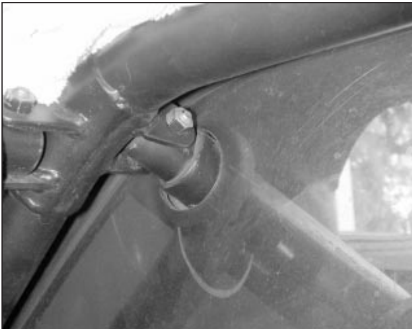
The bolt-in roll cage passes through the plexiglass rear window
