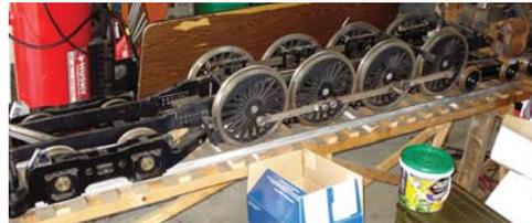
Mountain 4-8-4 Locomotive chassis. All wheels turned and mounted on frame. Some rods completed.
