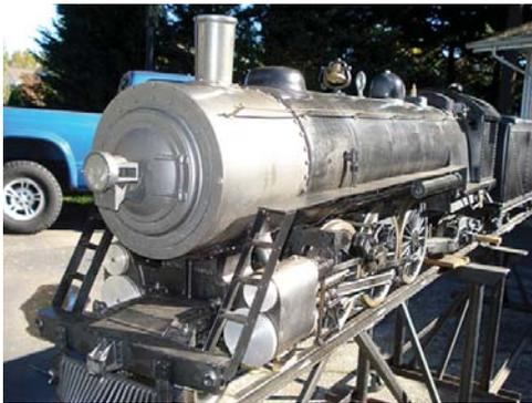
Pacific 4-6-2 Locomotive complete and running with prints. Passed all tests for 10 years. Steel boiler and tubes.
