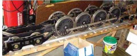
Mountain 4-8-4 Locomotive chassis. All wheels turned and mounted on frame. Some rods completed.
