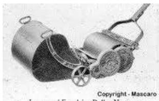
**Figure 1 A very early hand-powered Greens Mower.**
