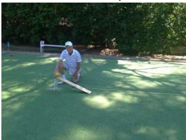
immersing himself in croquet.<sup>7</sup> What better person to develop a method for measuring the speed than a professor with a Cambridge doctorate in mathematics. And he made it remarkably simple! Prepare a 3 foot, 1”x6” board. Lay the board’s edge on the top of a croquet hoop (already a fixed height if set properly) and let the ball roll of its own weight from the highest point. Measure the
