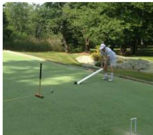
32x3/4”) and tightened it down in the center of the pipe. The idea, as in the Stimpmeter, was to place the croquet ball behind the bolt and then slowly raising the pipe until the ball releases. The pipe is held at that angle until the roll is finished. Bert Myer suggested it be a plain board affixed to the hoop height (to assure consistency). He playfully named this device “Bert’s Precision Ball Velociometer.” He said it could also double as a cribbage board!
