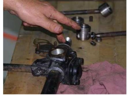
On the later models without lubrication nipples, the two covers just removed can be drilled and tapped for grease fittings. The covers are thick, but be sure that the fitting does not protrude into the working parts. Grease fittings are usually threaded ¼-28 and the proper tap drill is a #3, but a 7/32 makes the hole easier to tap and works fine.
