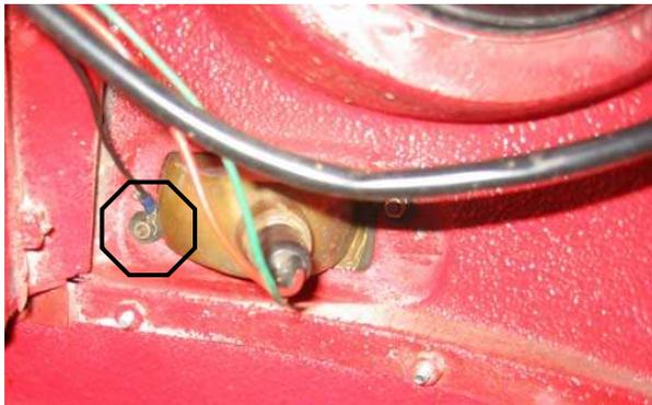
The forked or round connector goes over the bolt on the turn signal housing and is secured by the mounting nut (see octagon in picture) and the bullet connector goes to any black wire behind the grill. Make sure the connector at the housing is making contact with the nut, because some turn signal housings will have a rubber or plastic
