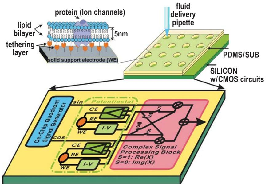
**Protein-embedded tBLM sensor arrays are built on top of the silicon surface; the electrical system underneath generates quadrature signals for two identical sensor elements, and the responses are processed in complex signal domain to get the real and imaginary portions of impedance information.**
