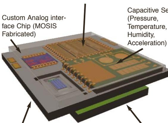
Silicon Platform with Chip Cavities, Microconnections, and Through-Wafer Interconnects
