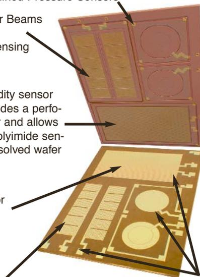
A MEMS chip measuring pressure, temperature, and relative humidity has been realized for an ultra-low-power environmental microsystem. The chip uses (1) a bimorph structure based on differential thermal expansion for sensing temperature and (2) a polymer structure based on moisture absorption for sensing relative humidity.
