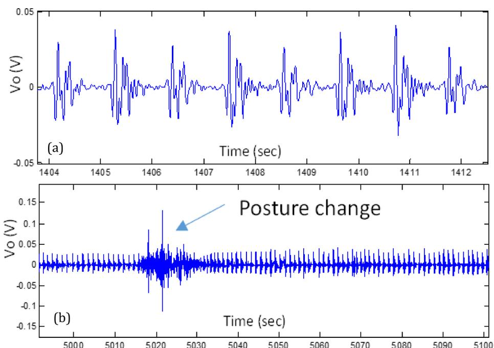
Fig. 2 (a) Enlarged view of BCG pulses; (b) large spikes caused by body movement.
