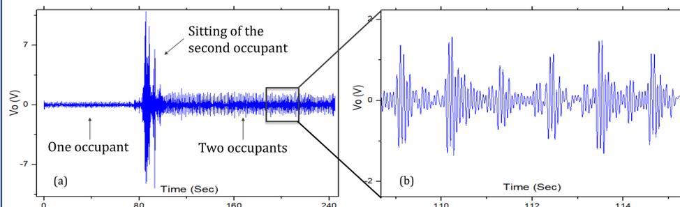
Fig. 4 (a) change of the BCG recording of one occupant to two occupants; (b) BCG signal recorded from two occupants in one bed simultaneously
