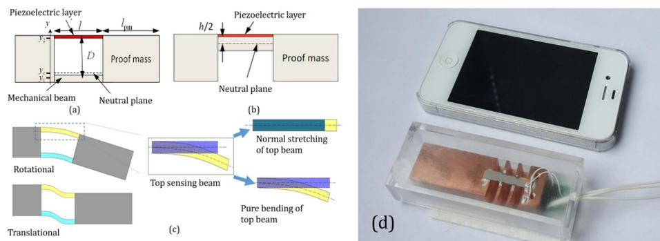
Fig. 1 (a) structure of accelerometer based on asymmetric-gapped cantilever; (b) structure of a conventional accelerometer; (c) decomposition of the bending of asymmetric-gapped cantilever; (d) an ultrasensitive accelerometer in comparison with an iPhone 4 smart phone.
