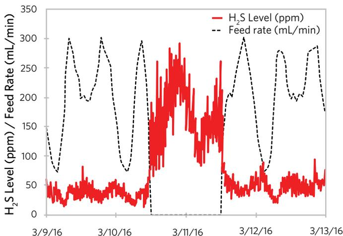
When the Alkagen AQ feed system was temporarily shut off, hydrogen sulfide levels spiked, demonstrating the effectiveness of the solution.
