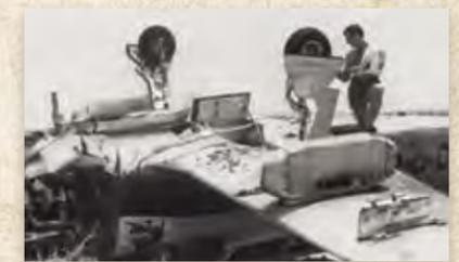
Top: Gear down off-field forced landings often resulted in aircraft flipping. This pilot only had minor arm injuries.
