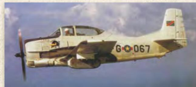
Look Ma, no tail hook! Tail hooks were removed, and cowl strakes were added to allow spin recovery with armaments on combat T-28Cs.
