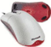
(The underside has a red light instead of a mouse ball), wipe it with a damp, lint-free cloth. Pay particular attention to the area from which the red light shines. No need to open up an optical mouse.
