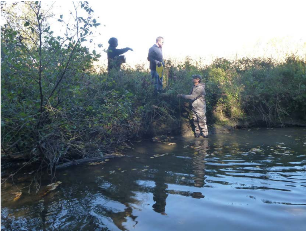
Caption: Jeff O'Handley, Chris Andreassen, and Mike Jura measuring stream banks for the Bank Erosion Hazard Index (BEHI) during the protocol training.
