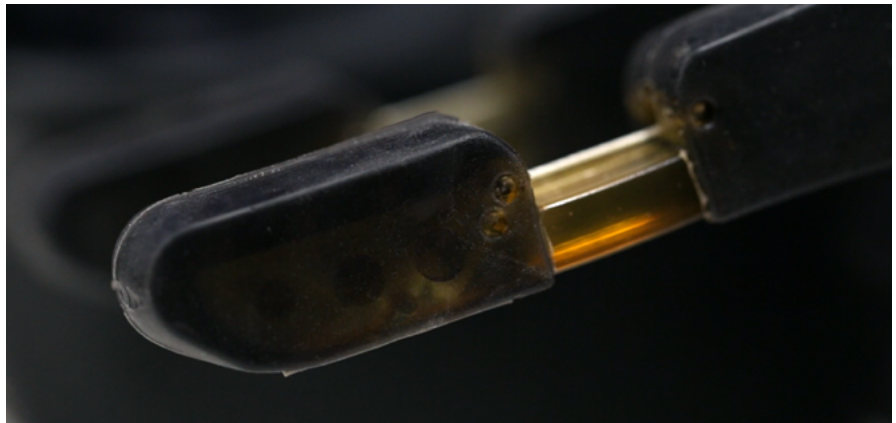
The outer layer gives the gripper enhanced tactile sensitivity and control, as well as sealing sensor electronics, through the use of softer low-durometer rubber.
