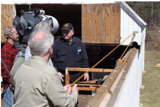
Testing the emergency roof closing system pulley. (L-R) Dave Prowten, John Maher, John Hinz, Steve Clougherty and John Blomquist. *
