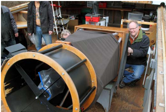
Phil Rounseville and crew working on the 25-inch Dob *
