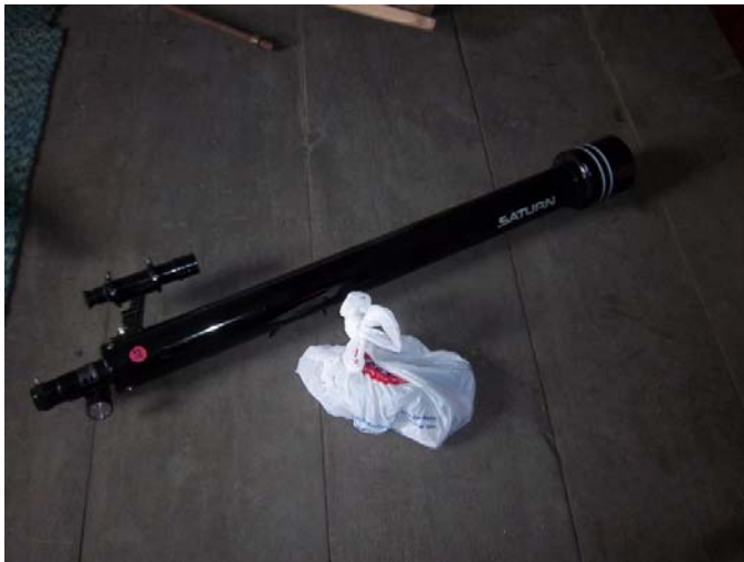
A25. Saturn Refractor. 60 mm, f/15
