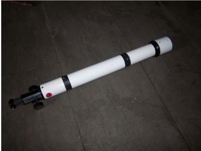
A18. Quality Optical Support Systems Refractor; 50 mm, f/12
