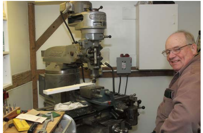
John Blomquist milling down the teflon block for the 25-inch base.*
