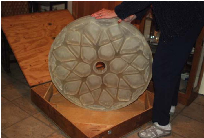
A lightweight 32-inch mirror blank
