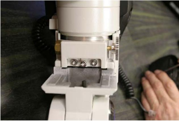
Check for end play on the shaft and make sure that the gear setscrew is tight and is positioned on the flat part of the shaft. The 3 hex screws that you see here are the worm adjusting screws.
