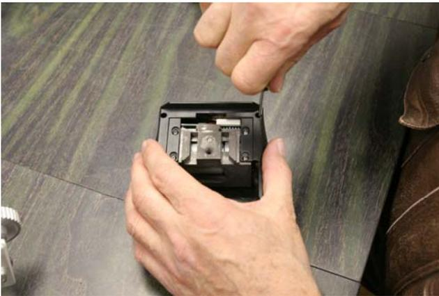
Using a small Phillips screwdriver remove the 4 screws that hold the housing in place.
