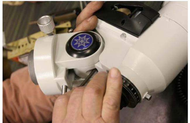
Remove the hex screw between the latitude adjusting screw and the polar scope.
