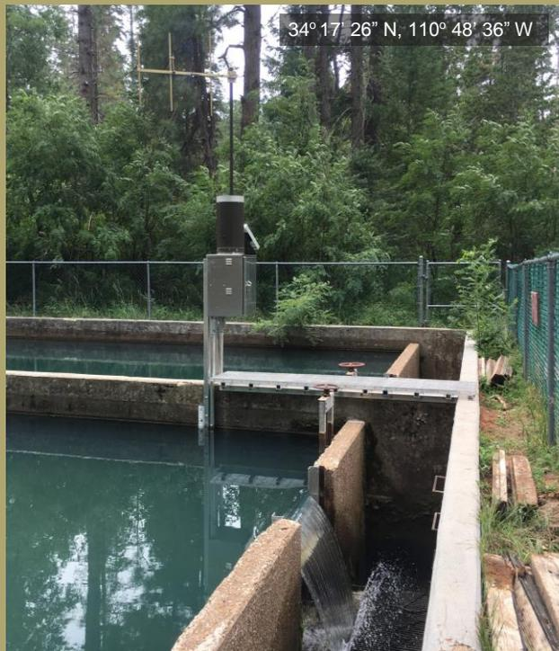
This new precipitation/ stream station was installed at the Canyon Creek Fish Hatchery, Arizona during August, 2016. This station plus other planned stations at the hatchery will use ALERT and cell networks to fulfill flood detection and data collection priorities.
