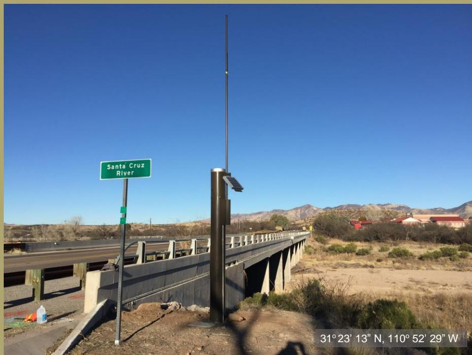
This ALERT precipitation and radar stage station was installed for Santa Cruz County on January 12, 2016 on the Santa Cruz River at State Highway 82 near Nogales, Arizona.
