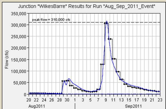
Figure 2 - Computed & Observed Flow Hydrographs at Wilkes Barre, PA
