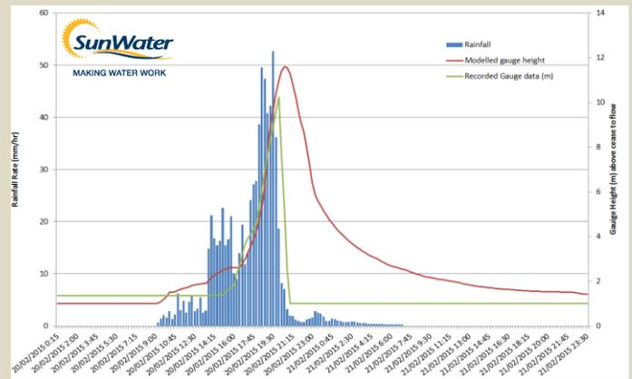
Figure 3: Catchment rainfall with river height and post event analysis from Callide Creek at ‘96k’.
