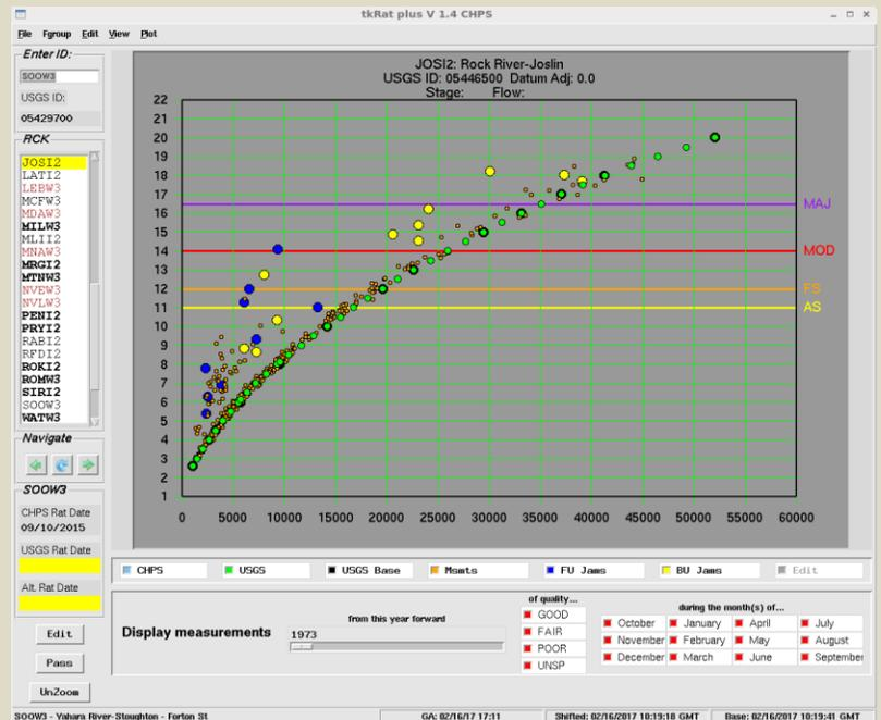
Figure 3: Plot with rating and ice jam events for Joslin, IL. Shifts of 1-6 feet due to ice have been observed.
