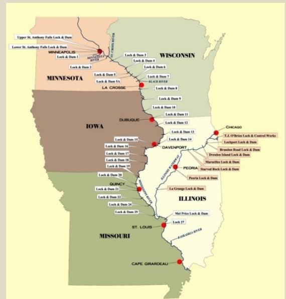
Figure 1: Upper Mississippi Basin Lock and Dam Structures
