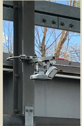
Radar stage sensor and surface velocity sensor
