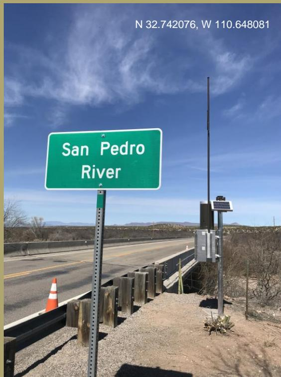
The Pinal County Flood Control District installed this new ALERT station on February 28<sup>th</sup> and March 4, 2019. Data from this and other stations in the Pinal County ALERT System can be accessed at:
