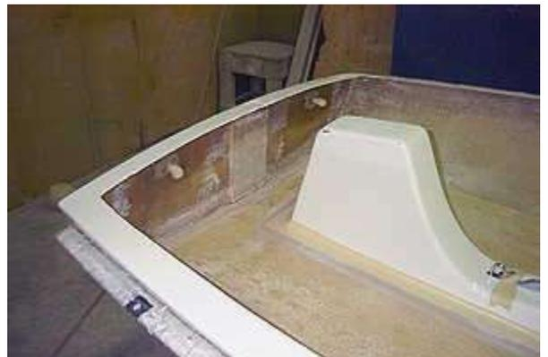
A look behind the bilgeboard box showing the reinforcements plus the aluminum plate for the board pivot bolt.
