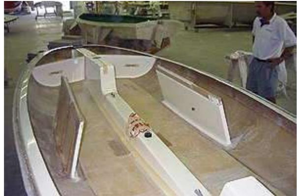
The mast step area of the strongback. Note the sidestay backing plate that has been glassed in underneath the edge of the hull.
