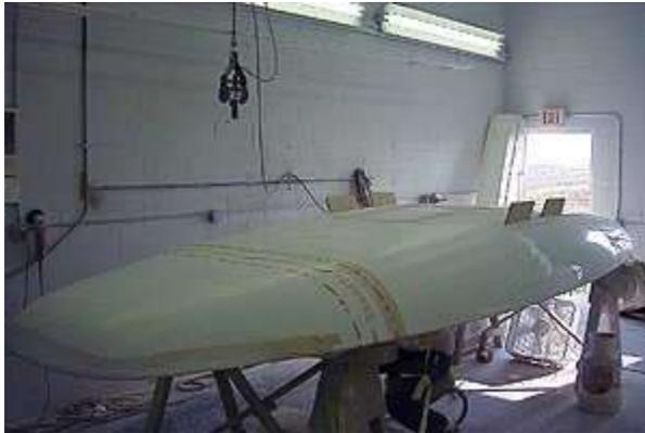
After the deck has been attached to the hull, it goes to the finishing area where blemishes are removed such as any center seam imperfections due to the clam shell mold. There is someone working under the hull!
