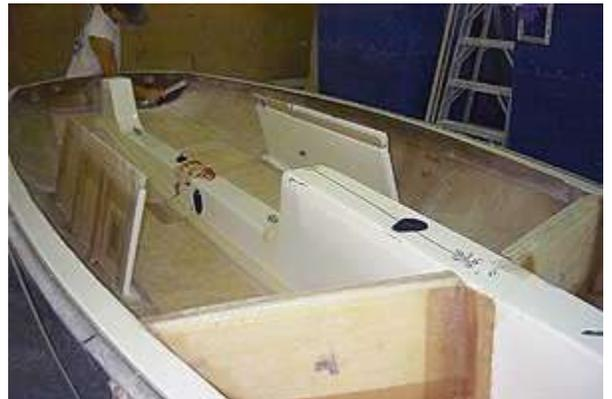
Note the reinforcements for the rudder gudgeons and the two blocks through which the shockcord runs that is attached to the board pull-down lines.
