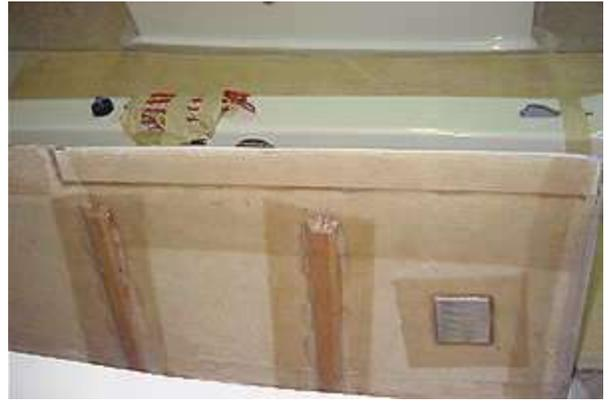
Note the core reinforced floor. Holes for the bailers have not yet been cut.
