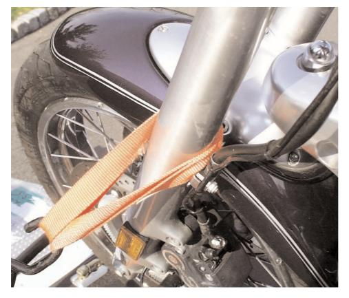
2. While one person remains on the motorcycle, attach straps around each of the front fork tubes just above the lower fork brace (refer to photo, note the position of straps). Do not place the motorcycle on the center or side stands.
