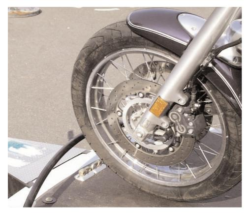
1. Begin the process by running the motorcycle onto the trailer with the front wheel firmly against the wheel chock. The suggested method of tying the motorcycle down is to have one person sitting on the motorcycle with the other attaching and tightening the tie-down straps. The person sitting on the bike should remain seated until the front tie-downs are both attached and fully tightened.
